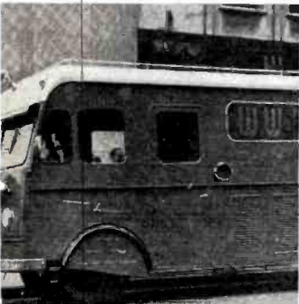
NEW remote truck of WWJ-TV Detroit, custom made to WWJ's specifications by the Ketels Mfg. Co., was delivered last month and used day following receipt at a baseball telecast from Briggs Stadium. Painted a fire engine red, the truck is 25 ft. long, 9 ft. 6 in. high and 8 ft wide.
