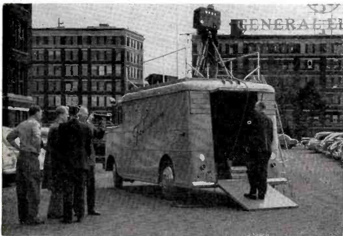
BEFORE installation in the camera atop WGRB (TV)'s mobile unit, a telescopic lens is inspected by GE's television technicians. The mobile transmitter has telecast more than 30 "remote" shows in its first year of service for WRGB (TV). A crew of seven includes two cameramen, three controlmen, a program director and an announcer.
