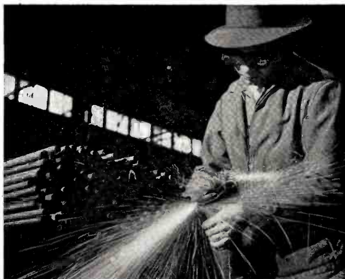
3 CAN YOU "READ" SPARKS? This man is testing scrap steel for alloy content. He can identify many alloy steels by shape and color of sparks. Identification is important because wrong alloys can affect whole furnace charge.
