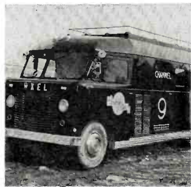
Remote truck has its own 10 kw generator, RCA microwave transmitter, three camera chains plus Zoomar lens. It's air-conditioned.
