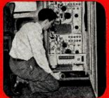
✓ Convenient, accessible rack unit. 2-way telephone communication between rack, camera and control console.
