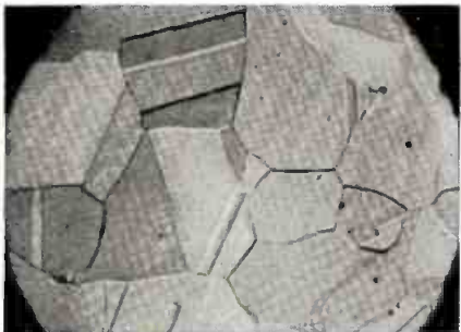
3. Here is a micro-view of a highly alloyed steel in its toughest state.
