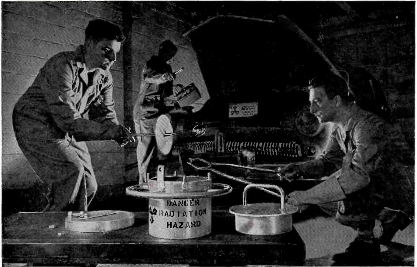
PISTON RING MADE RADIOACTIVE in Atomic Pile at Oak Ridge, is carefully installed in test car engine by specially trained scientists. Radioactivity is checked with Geiger counter at all times. Car is then driven in proving
