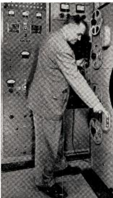
An Ampex Automatic Station now in operation at KEAR in San Mateo, California. It sustains the evening programs on tapes prepared by the daytime staff.
