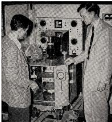
INSPECTING the roll-out dolly which houses tuning coils and the Klystron amplifier for DuMont's 5 kw uhf transmitter built for WNOK-TV Columbia, S. C., are Stan Pauloski, research engineer for DuMont, and Don Willoughby, chief engineer for WNOK-TV. The Columbia station is assigned uhf Ch. 67 and began operating Sept. 1.
