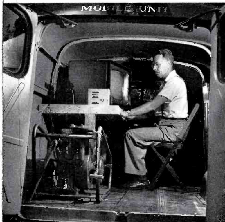
WEEU-TV, Reading, Pa. Harold E. Schearer, Asst. Dir. of Tech. Operations, uses equipment in the station's mobile unit to measure the field strength of the broadcast signal from any given point within the wide radius of the station's transmitter.
