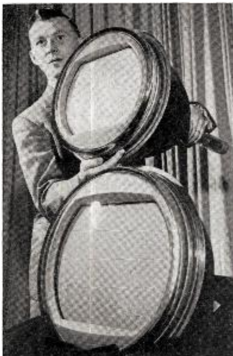
NEW RCA developmental 19-inch color tube is compared with the current 15-inch color tube by Dr. D. Joseph Donahue, development engineer of the RCA tube plant, Lancaster, Pa. Area of the new tube nearly doubles the 15-incher.
