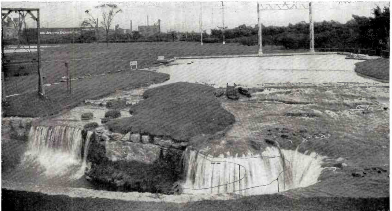
Large outdoor model of Niagara Falls, developed over 30 years ago by the local electric company, helped determine
