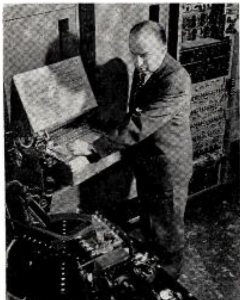
THIS IS RCA's "Electron Music Synthesizer," new instrument which synthesizes familiar sounds and, according to Dr. Harry F. Olson, seen operating the keyboard of the machine at RCA's labs in Princeton, N. J., creates an unlimited range of tone variations. It reportedly has "a capacity for originating endless varieties of rhythms."
