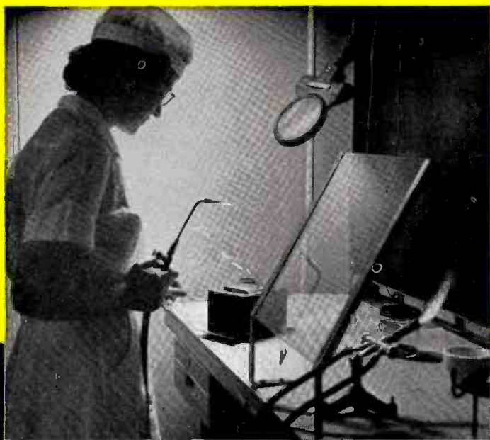
G-E quality methods in building Broadcast-Designed camera tubes, are shown by the care with which this glass technician fabricates an image-orthicon target. The glass bubble she holds is only 1/10,000 inch thick. After cutting out a small section, she must seal this to a metal ring. Any false movement would completely ruin the fragile target.
