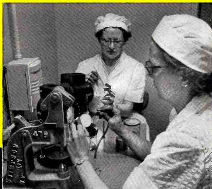
Dust and lint are banned. Note the lint-free Nylon uniforms worn by these skilled G-E workers while assembling the target and mesh for a Broadcast-Designed camera tube! In addition, the air is filtered and conditioned. A single particle of dust in the 1/500-inch spacing between target and mesh could mar tube quality, causing rejection.
