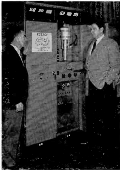
EXAMINING Philco's low-power tv broadcasting equipment are S. C. Spielman (l), director of electronic engineering, and James D. McLean, vice president of the company's Government & Industrial Div.
