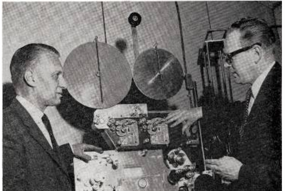
HOWARD L. KANY (left), manager of newsfilm, CBS News, nears from inventor R. C. Rheineck , chief engineer, CBS News, how this custom-built prototype of a magnetic stripe film printer operates at Du Art Film Labs., New York. Mr. Rheineck's right hand is pointing to assembly which makes magnetic print directly from magnetic original (both film picture and magnetic sound stripe). Assembly below this makes regular optical sound-and-picture print from magnetic original.
