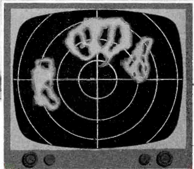
Black holes inside the white show areas of heaviest precipitation. Hooked finger formation indicates tornado funnel.
