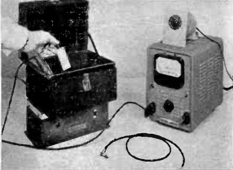
Test factually demonstrates shielding effectiveness of Netic alloy material and enclosure design. Instrumentation used: magnetic field radiating source, AC vacuum tube voltmeter, Variac, pickup probe and Netic Tape Data Preserver. For complete test details and results, request Data Sheet 142.
