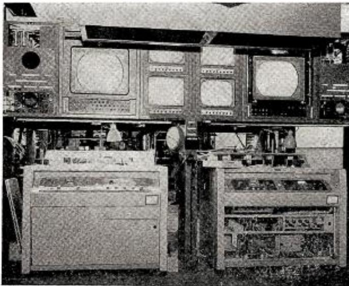
Color videobay • This section includes a pair of color video tape recorders. Grills directly above the vtr's are audio speakers for each of the two consoles. Price Fish, of the New York engineering staff, was responsible for much of the design work on the center and supervised equipment installation together with CBS-TV's west coast staff headed by Les Bowman.
