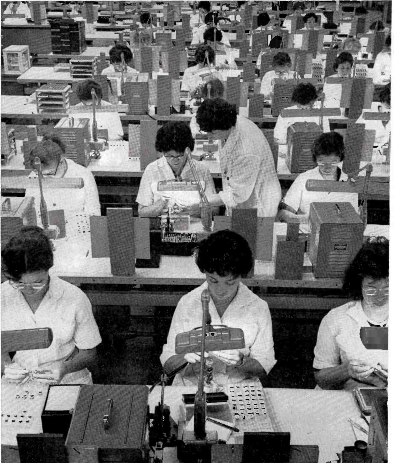
"SNOW WHITES" are girls at Western Electric's new Kansas City Works who work in super-clean conditions to produce miniature electronic products for the Bell Telephone System to the most exacting specifications. The girls you see are assembling mounts for electron tubes which will be used in Bell System telephone amplifiers.
