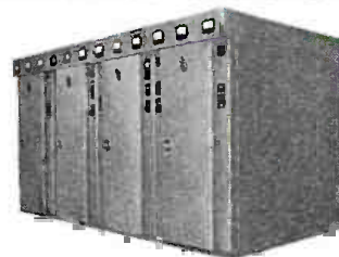
Type 317B 50kw AM transmitter
