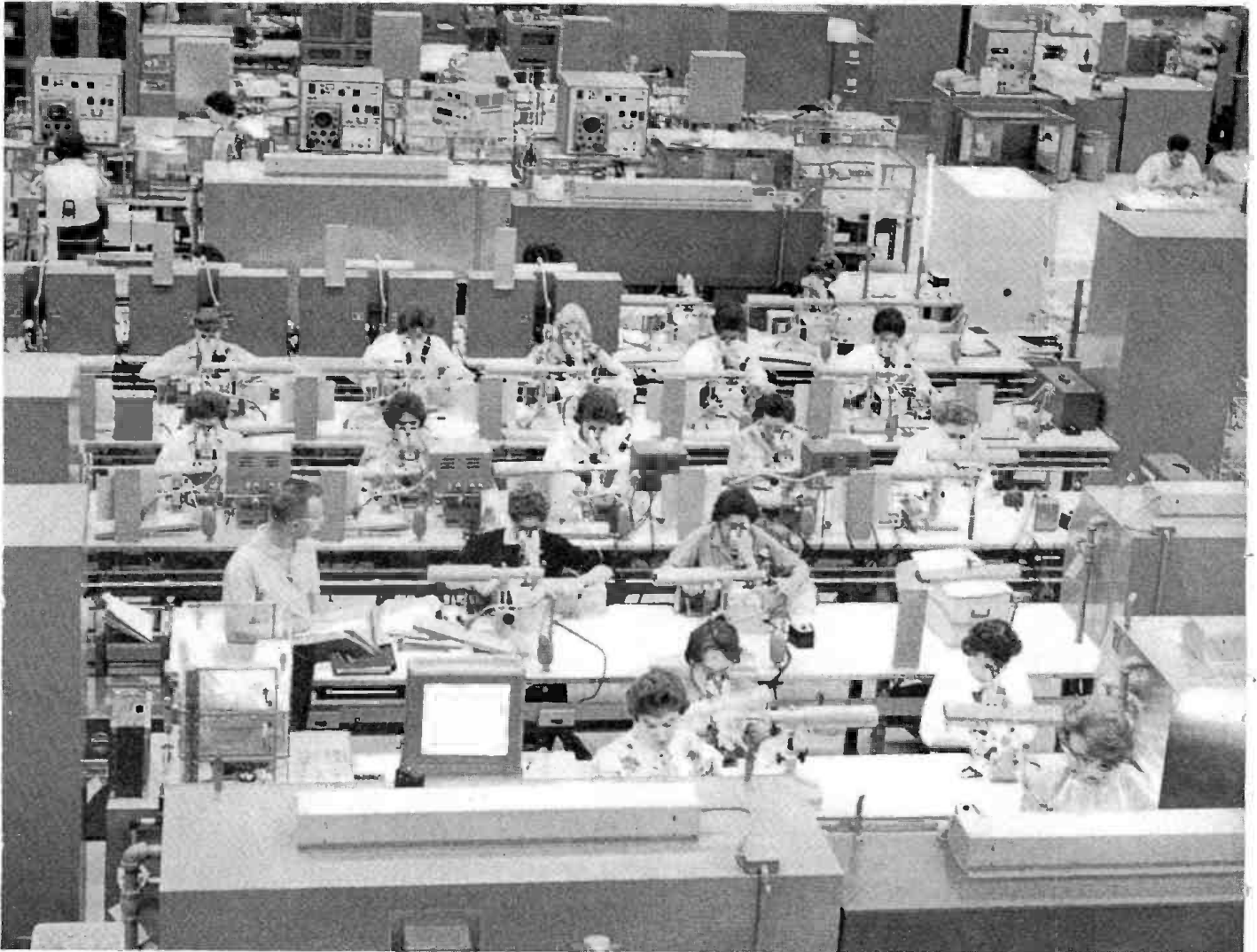
NIMBLE-FINGERED girls assemble tiny transistors under clean conditions at Western Electric's Allentown Works. The transistor, an invention of our research team-mate, Bell Telephone Laboratories, and dozens of other Allentown Works products play a vital role in the complex 65-million-telephone Bell System network.
