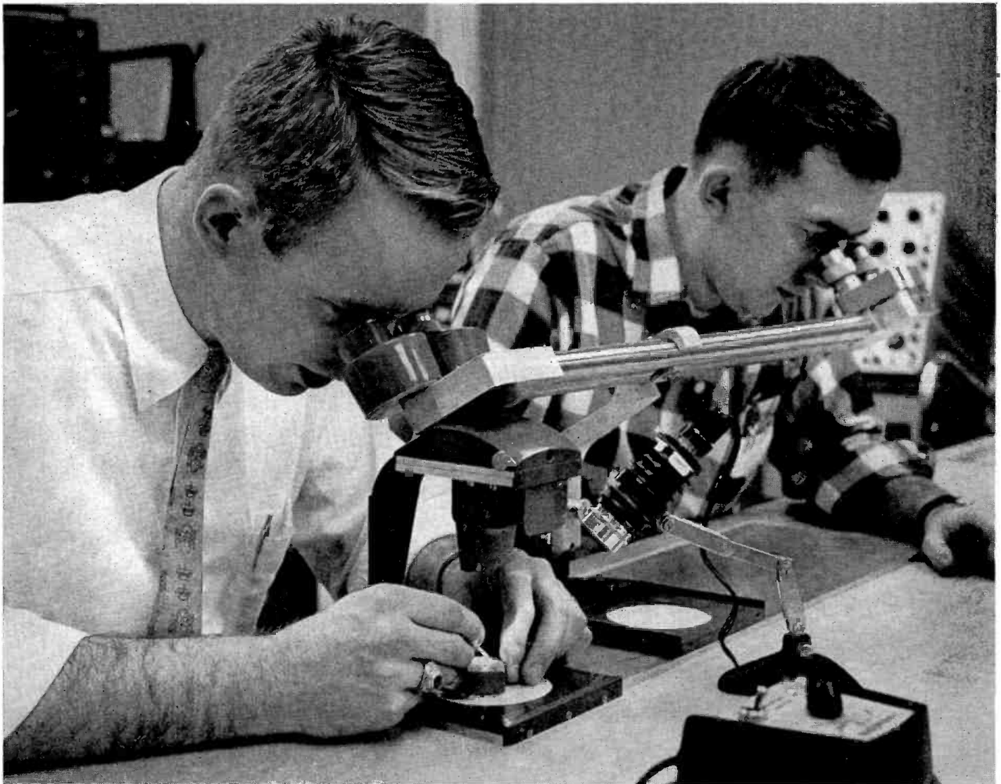
New Trainee Stereo Microscope was developed at the Engineering Research Center by Richard Dyer, a Research Engineer. Two sets of eyepieces and an intricate optical system allow two people to examine an object simultaneously and see an identical view. The trainee microscope provides an efficient, economical way to instruct W.E. plant personnel in the assembly of transistors and other solid state devices. Richard Dyer, left, tries out the scope with Technical Assistant Ronald Carter.
