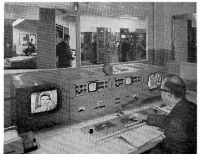
Administrative and technical supervision over video-tape and film facilities, some of which can be seen through the windows, is maintained from the 'central operations command post.' Technician monitors output of tape machine.
