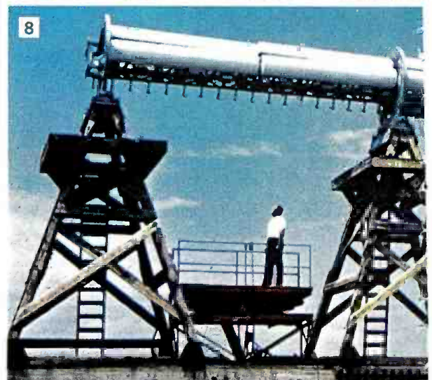
(8) Giant turntable called "Tiny Tim" where test antennas up to 15 tons move on a circular track 90 feet in diameter. It is one of three large turntables available for testing.
