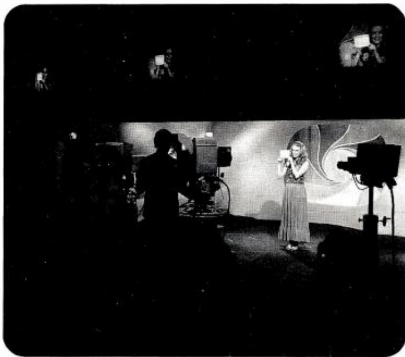
A look at a white card or any white area of a scene allows the cameraman to automatically adjust TK-44B white balance for consistent scene-to-scene colorimetry.
