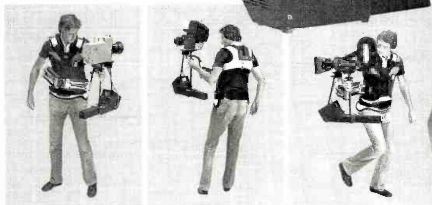
"Universal Model" STEADICAM shown in use with TK-76 video camera, CP-16R 16mm camera and CP-modified Arri IIC 35mm camera. Other video and film cameras of the same general weight class can also be adapted for use with the STEADICAM system. For further information, please write to:
