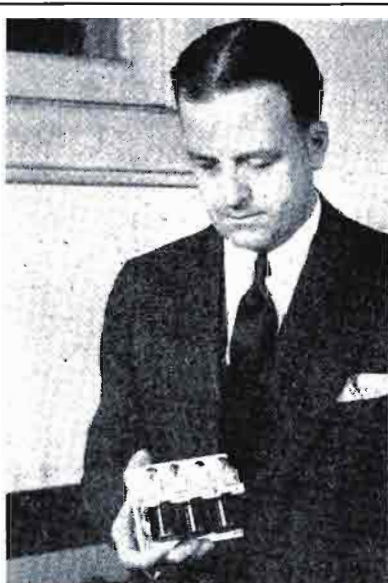
POPPEL'S LATEST —Jack Poppe, WOR chief engineer, recently elected to the board of directors as well as secretary of Bamberger Broadcasting Service, devised this midget microphone preamplifier for the Democratic convention. It weighs less than three pounds, measures less than 5 inches the longest way, has a net gain of 90 db, provides a linear response from 20 to 20,000 cycles and combines a two-circuit mixer with a three-stage, audiofrequency amplifier. It incorporates new AmerTran midget audio transformers and RCA acorn tubes.
