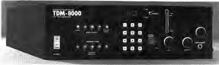
The old squeeze play. Time compression and expansion devices allow broadcasters and producers to speed up or slow down the running time of programs or commercials without creating disturbing pitch distortion in the audio. The Eventide Clockworks system (top) is capable of both compression and expansion; Integrated Sound Systems' box (below) is capable of compression only.
