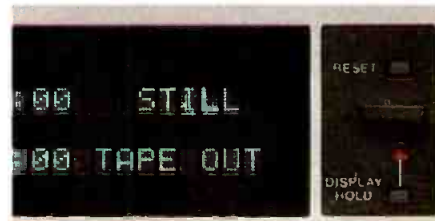
Display board for self-diagnostics and other data-processing functions.
