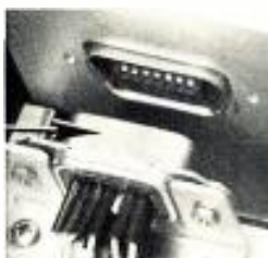
All deck leads go through this plug-in connector . . . nothing to disconnect to remove deck.
