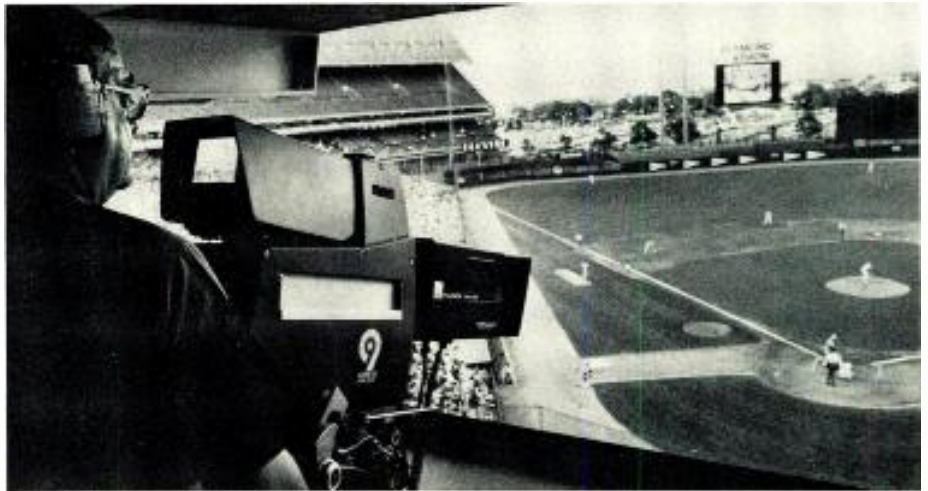
Channel 9 covers home plate action from one of their six TK-47 automatic color cameras. In the distance, the Met's Diamond Vision replays game action in slow motion from another TK-47 output.
