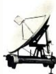
Our 3.66-meter audio-only uplink. The electronics are housed in rugged carrying cases that are easily transported and quickly set up.
