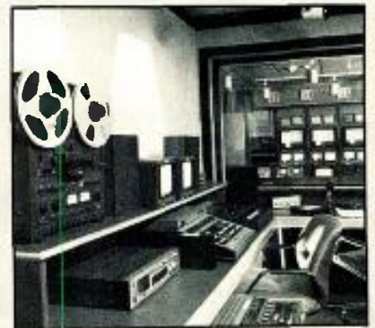
Redmen television. The broadcast booth and control room shown above are part of a new $3-million television center opened at St. John's University in November. The facility, designed for the use of 700 communication majors at the Jamaica, N.Y., institution, is outfitted with broadcast quality gear including three Ikegami studio cameras and separate field cameras, Sony one-inch studio videotape recorders and portable U-Matics with a Sony BVE-5000 editing system, a Chyron character generator with a color palette feature, a GVG 300 production switcher, an NEC digital video effects system, an MCI audio board, and a Strand Century lighting system. The center will be directed by Patricia Ruggieri, former operations manager of the Center for Non-Broadcast Television Inc. New York.
