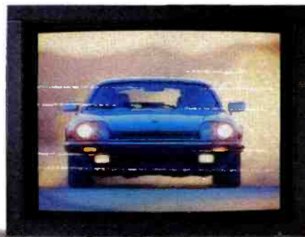
With a Variable Cut system, tape wear can become a visible problem.
