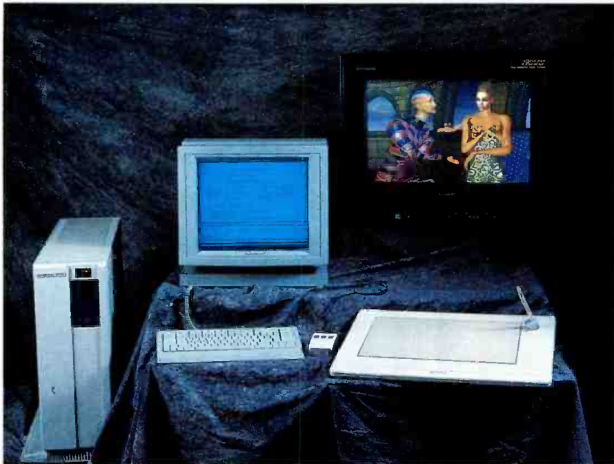
Symbolics HD XL Animation, like PALTEX EDDi, is integrating paint and 2D and 3D animation tools in PC-based systems able to capture multiple formats, including HDTV.
