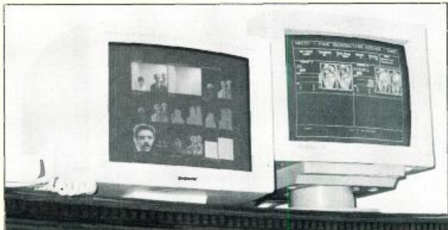
These two screens demonstrate the computer imaging process that will take place inside the passive meter box in the home; the system will create and store data allowing it to identify individual viewers in a room
