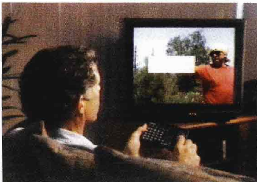
A prototype of VideoFreedom obscuring technology demonstrates how a TV set can block out a specific portion of the screen. In this case, the man on the screen is holding a gun, but the system can be used to block any or all parts of a scene.
