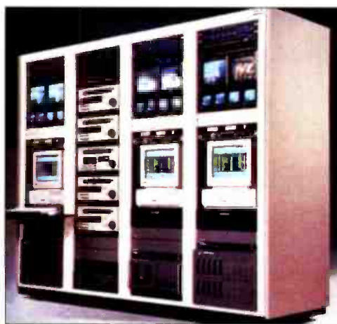
Odetics' Spotbank automation system uses a disk-based server for storage of all commercial and spot inventory.
