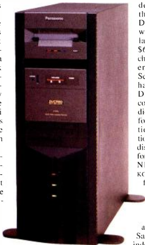
Panasonic's DVCPRO mini-tower nonlinear editing workstation features a built-in DVCPRO VTR and disk transfers at four times faster than real time.
