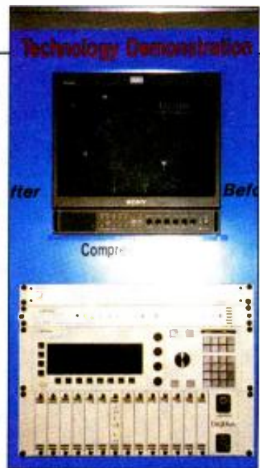
Leitch's MPEG-2 compression system supports both 4:2:0 and 4:2:2 encoding.
