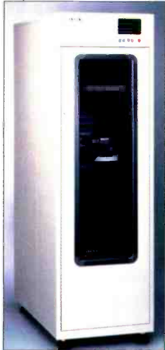
Channel Earth uses a Sony Flexicart robotic tape handler.
