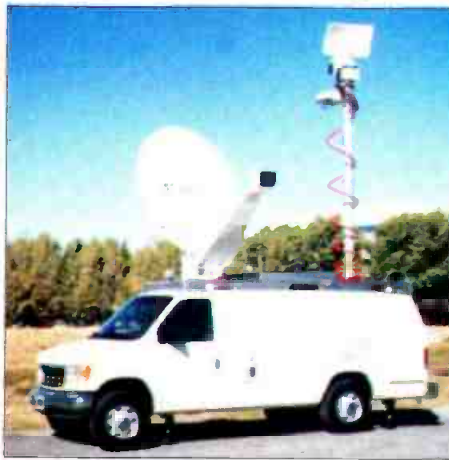
ENG Mobile Systems' OmniLink 2000 van has both ENG and SNG capabilities, including a 30-foot microwave mast and 1.8 meter satellite antenna.
