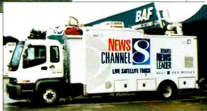
A large 'combo' truck BAF built for CBS affiliate kcci(tv) Des Moines, Iowa. The SNV-210T dual-path SNG truck has a 42-foot microwave mast.
