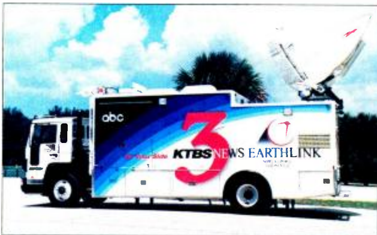
Frontline still advocates big SNG trucks for customers who need them, such as this analog 'Super Truck' Ku-band unit it built for ABC affiliate KTBS-TV Shreveport, Ala.
