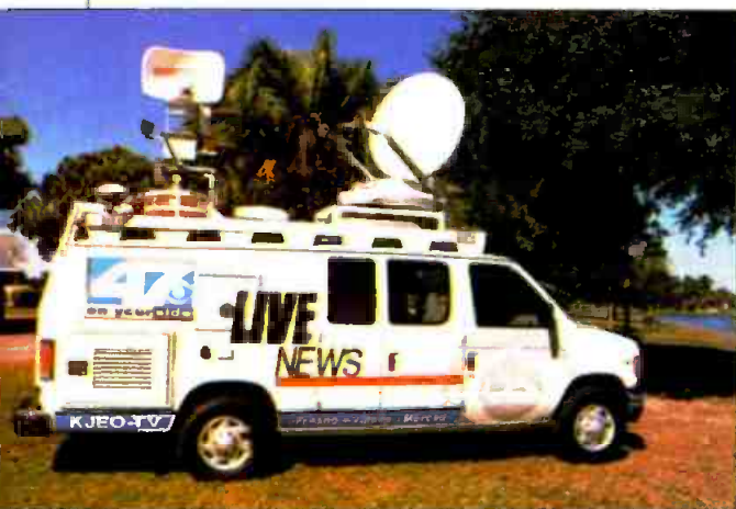
A combination microwave SNG van built by Frontline Communications for CBS affiliate KJEO-TV, Fresno, Calif.
