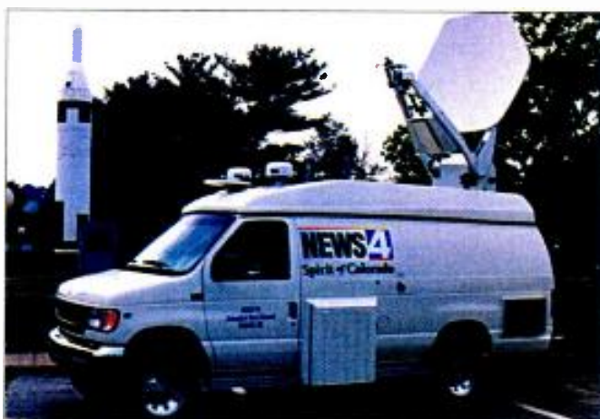
Wolf Coach built this digital Ku-band van for CBS O&O KCNC-TV Denver. The van has a lightweight 1.5-meter carbon fiber antenna and Tiernan MPEG-2 compression gear.
