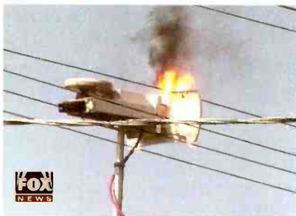
When the mast on KABC-TV's electronic news-gathering van hit a power line, the microwave antenna exploded.
