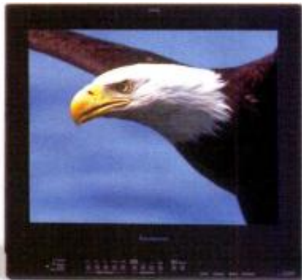
Panasonic's 18-inch BT-LH1800 is an LCD monitor that incorporates CRT features.
