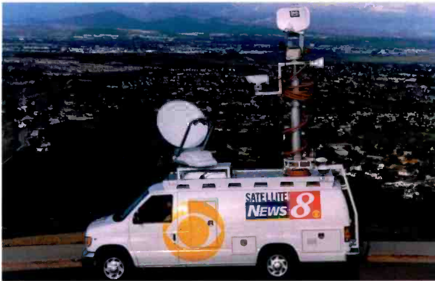
Recommended codes for newsgathering vans would require training, equipment and inspections to prevent injuries—especially those caused by contact with overhead electrical wires.
