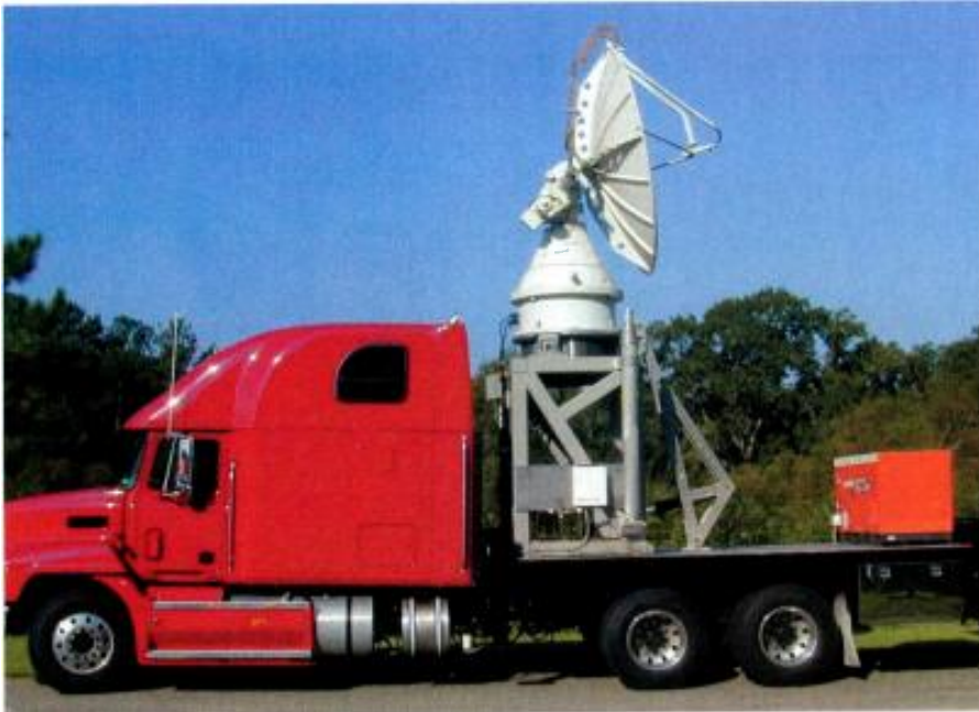
FSU's mobile radar truck weighs 35,000 pounds and can withstand a Category Five hurricane.
