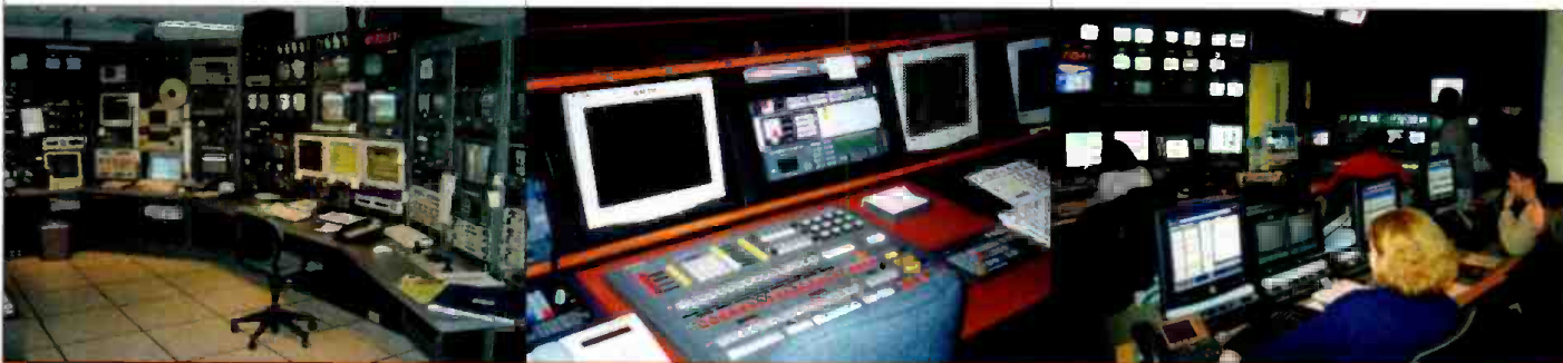
Automation has reshaped news operations like Chicagoland (left), with a Harris system, and NY1 (right), with an Omnibus setup. Public broadcaster WNET(TV) New York (center) has improved operations with a Harris automation system (originally installed as a Louth system).
