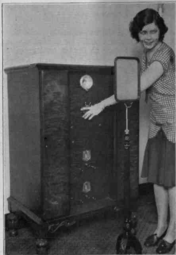
The television console shown here holds two receiving sets, one for sight and one for sound, a loud speaker and a televisor, also a screen on which the picture appears.
