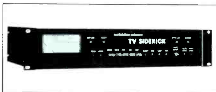
This black box, which adds SAP to a TV station's signal, is in short supply.
