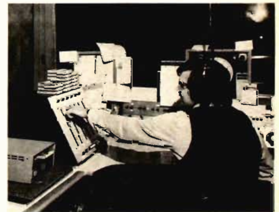
Example of a semi-automated, semi-manual system, where the announcer sets the programming sequence for the next 15 minutes.
