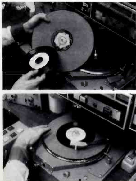
FIG. 3A and 3B SLIP CUEING DEVICE
