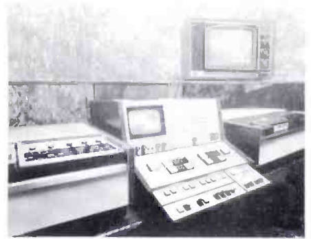
OFF-LINE EDITING. Rapid search with time code reference saves hours and money, making on-line editing faster and more efficient.
