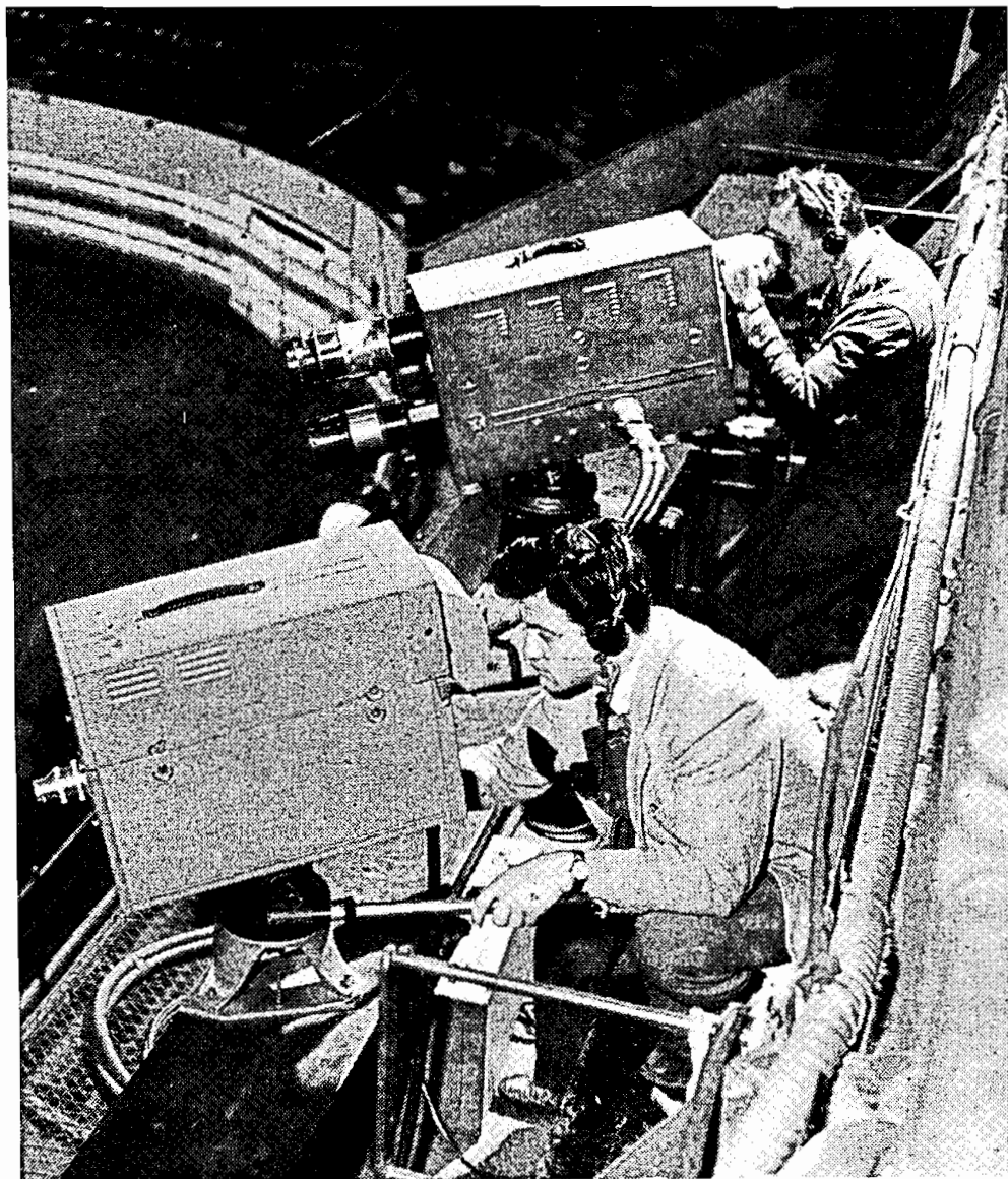
RCA's new super sensitive television camera (foreground) was placed along side the conventional camera at Madison Square Garden, New York, recently, in a demonstration of the new camera's improvements. The new camera displayed a greater depth of perception and clearer view under imperfect lighting conditions.
